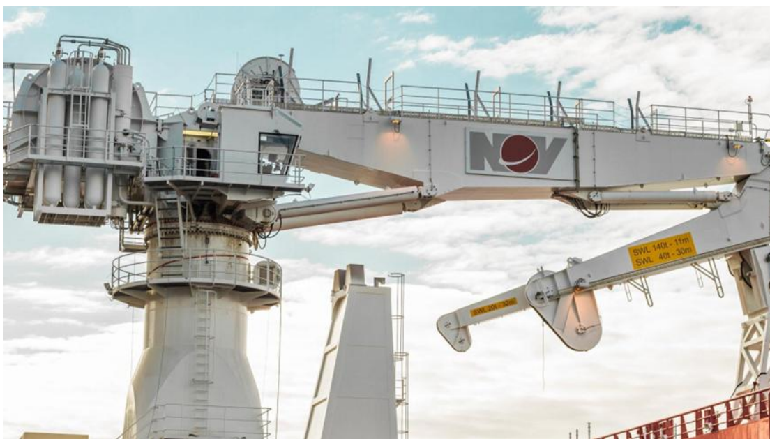
Slika 44 – Brodska dizalica SWL 140 T (Offshore crane National Oilwell Varco)
